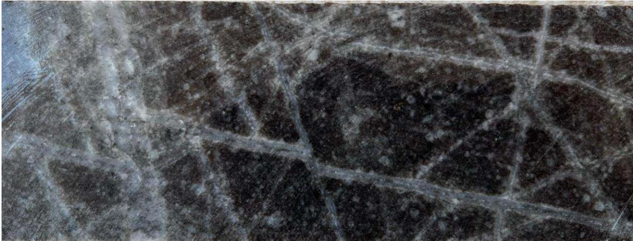
Figure 1 – Hole LM24DD001 at 239.2 meters. Biotite-altered monzonite with (1) sinuous quartz, (2) quartz-sericite-pyrrhotite-chalcopyrite, (3) quartz-pyrrhotite-chalcopyrite, (4) irregular quartz-pyrrhotite-chalcopyrite-pyrite-molybdenite (sericite selvage), and (5) sinuous quartz-sericite veinlets and disseminated chalcopyrite.
