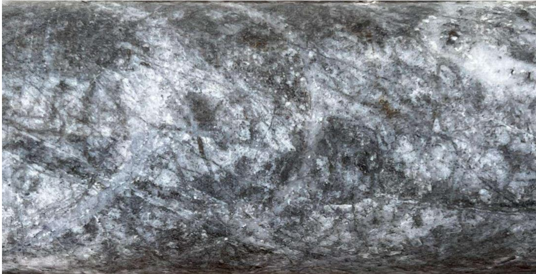
Figure 3 – Hole LM24DD002 at 65.90 meters. Biotite-altered Hornblende monzonite with overprinted quartz-sericite ± chlorite alteration. Stockworking is constituted by quartz-pyrrhotite-molybdenite, pyrite-chalcopyrite-molybdenite and quartz-pyrrhotite-molybdenite veining.
