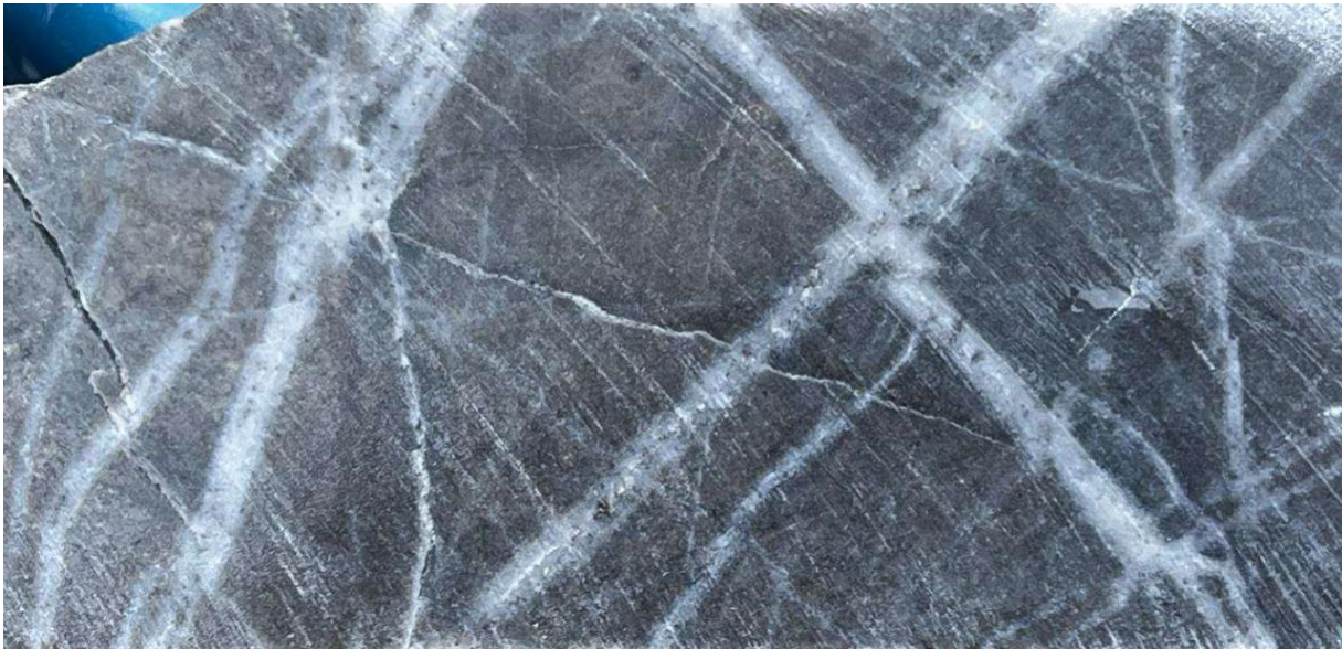
Figure 2 – Hole LM24DD001 at 265 meters. Biotite-altered slate with quartz-pyrrhotite-molybdenite-chalcopyrite veining and disseminated chalcopyrite.
